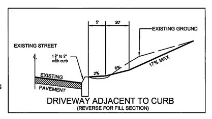
ALL CHANGES IN VERTICAL GRADES SHALL BE MADE WITH SMOOTH VERTICAL CURVES NOT LESS THAN 25' IN LENGTH.
